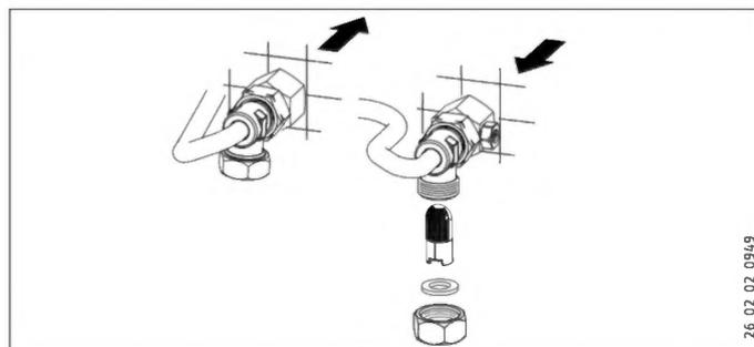
If dirty, clean the strainer in the threaded cold water fitting. Close the shut-off valve in the cold water inlet line before removing, cleaning and refitting the strainer.
